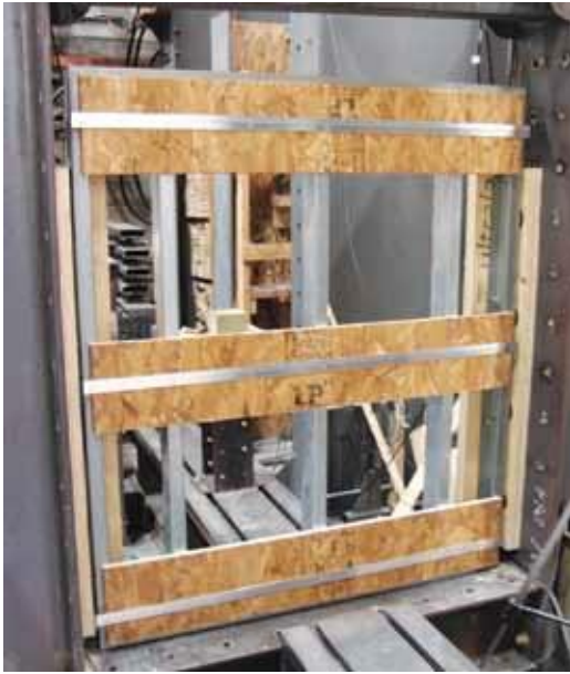
Figure 7: Test Set-up 2 – Wall Mount
